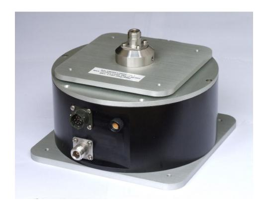
The RT6 is a single axis rotating platform capable of traversing loads up to 20 kilograms, such as offset dish and large patch antennas. The output disc can be continuously rotated through 360 degrees through the internal microwave R.F. slip-ring assembly. The functions of the RT6 are controlled remotely through a bi-directional RS485 interface.
